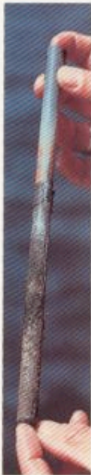
Figure 7-5. As evidence of the high temperatures present in the black smokers, consider this Alvin heat probe, which was inserted into the smoke to measure its temperature. The hottest waters ever encountered prior to the black smokers were 22°C, so not only did the temperature reading from this probe go off the scale, but the PVC plastic tubing melted. Melting temperature for PVC is 250°C. High-temperature platinum thermocouples were later used to measure temperatures up to 400°C in the black smokers (by Emory Kristof, © National Geographic Society).
